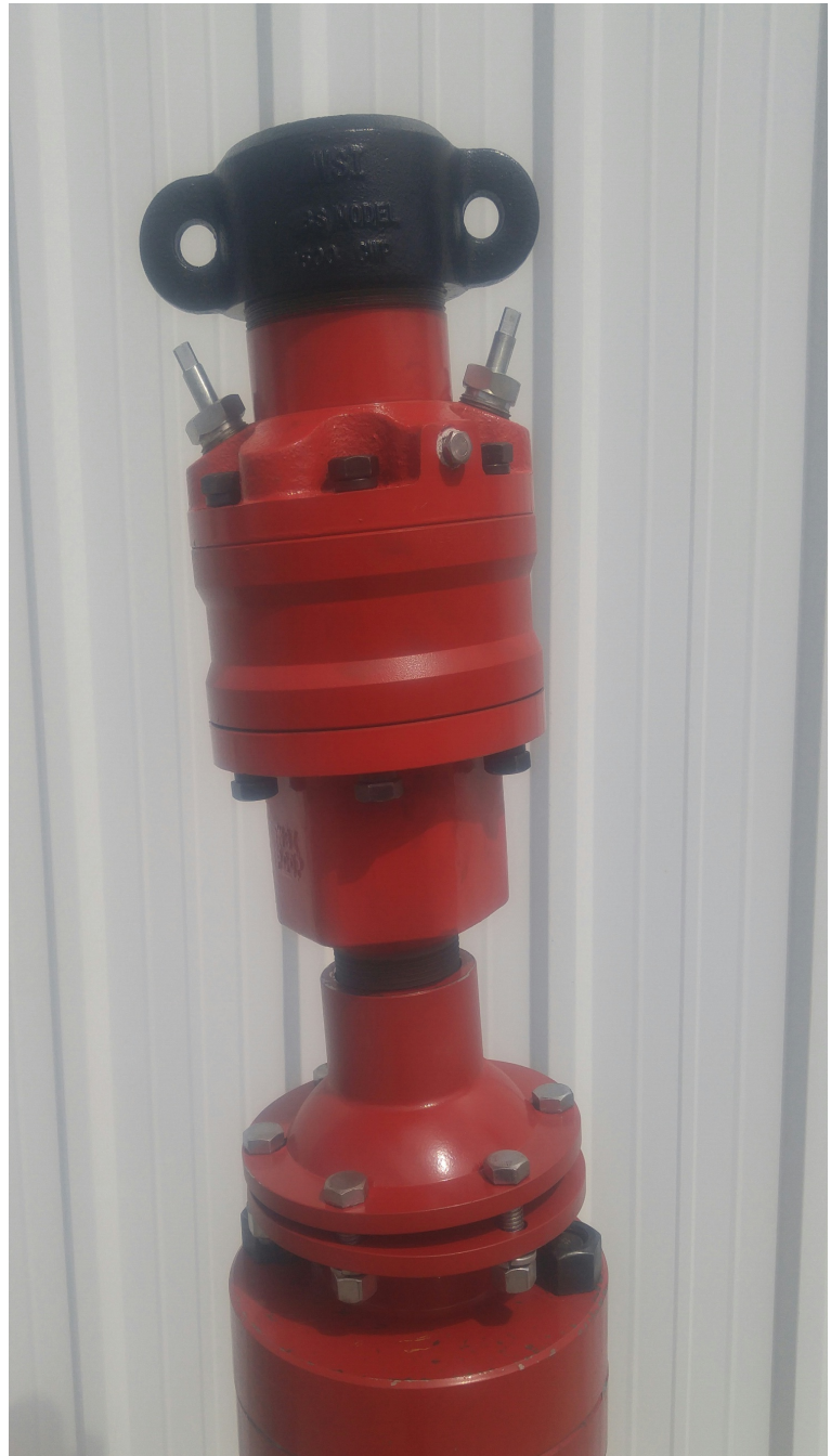
1500# Model "BS" PCDP on Misalignment Tool, with adjustment to the alignment of Stuffing Box
