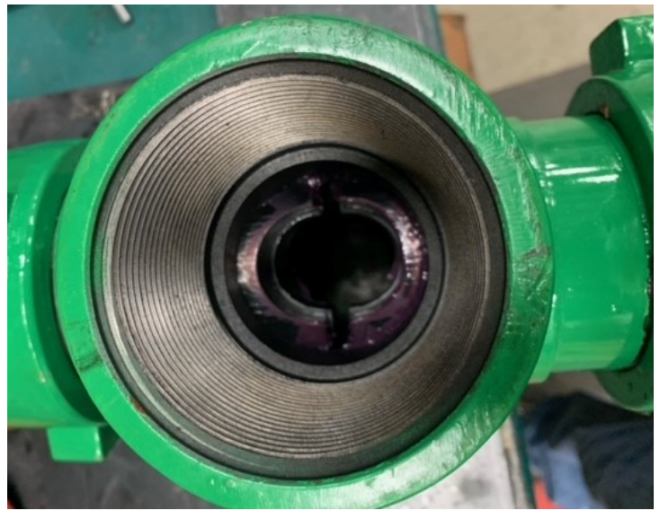
After, ram aligned with polish rod to vertical position
