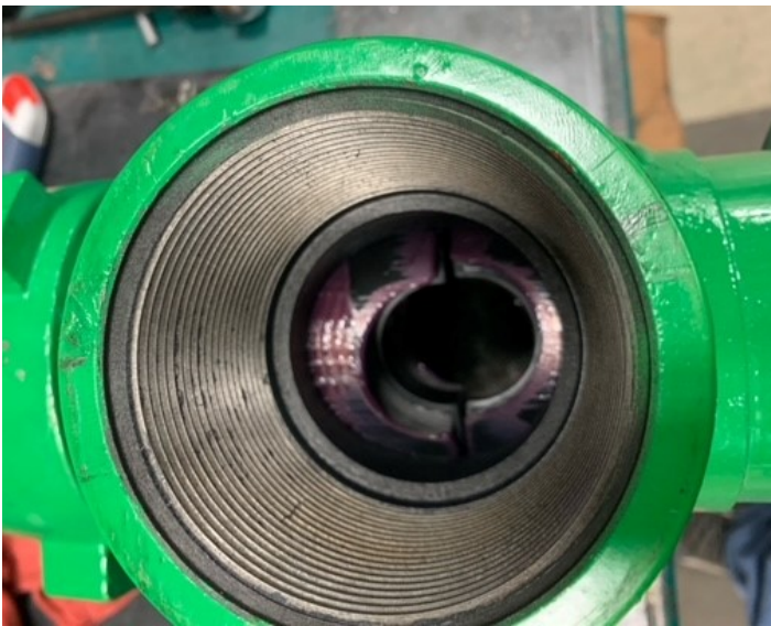
Before, ram on the right is off center
